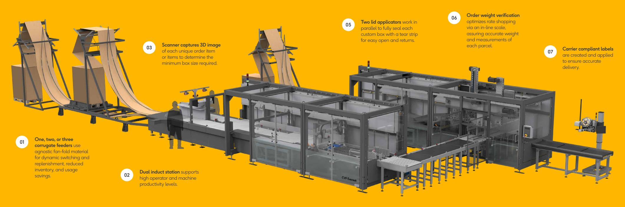
Case erector builts a fit-tosize box bottom and allows for a wide range of sizes.
